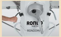
As an option, the Rondomat is available with a reversing lever. This is practical when you stand adjacent to the machine to get a better view of the dough band.
