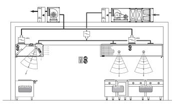
The cooking equipment is gradually heated according to the requirements of the menus to be prepared. The IRIS sensors associated with temperature sensors detect the state of the equipment concerned (hot and in hold). The system then automatically adjusts the position of each individual damper and the fan speed, in order to achieve the exact flow rate required for each hood in response to changing requirements.
