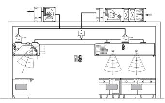
When the galley is not in operation, M.A.R.V.E.L. can be programmed to stop the ventilation or to continue it at a low flow rate that keeps proper hygiene maintained during the inactivity. In the latter case, the fans and dampers are automatically adjusted to the minimum programmed settings.
