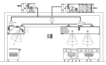
The cooking equipment is gradually heated according to the requirements of the menus to be prepared. The IRIS<sup>™</sup> sensors associated with temperature sensors detect the state of the equipment concerned (hot and in hold). The system then automatically adjusts the position of each individual damper and the fan speed, in order to achieve the exact flow rate required for each hood in response to changing requirements.
