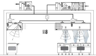
When the galley is fully active, most of the equipment enters cooking mode while the other equipment generally remains on standby. The infrared sensors once again detect this change in activity, as it occurs. The exhaust (and fan) flow rate is then automatically adapted to the change in requirements, hood by hood in real time.
