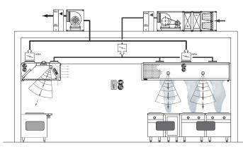
When the galley is fully active, most of the equipment enters cooking mode while the other equipment generally remains on standby. The infrared sensors once again detect this change in activity, as it occurs. The exhaust (and fan) flow rate is then automatically adapted to the change in requirements, hood by hood in real time.
