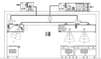
When the galley is not in operation, M.A.R.V.E.L. can be programmed to stop the ventilation or to continue it at a low flow rate that keeps proper hygiene maintained during the inactivity. In the latter case, the fans and dampers are automatically adjusted to the minimum programmed settings.
