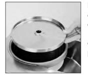
Next, fit the corresponding slicing disc (straightedged blade) and rotate in a clockwise direction to ensure that it is correctly positioned.
