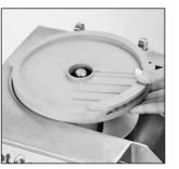
Next fit the appropriate slicing disc and rotate in a clockwise direction to check that it i correctly positioned.
