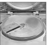
3) Position the head of the vegetable preparation machine on the motor shaft. The fastening hook should now be facing you, on your right.
