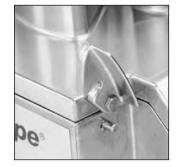
4) Position the head of the vegetable preparation machine on the motor shaft. The fastening hook should now be facing you, on your right.
